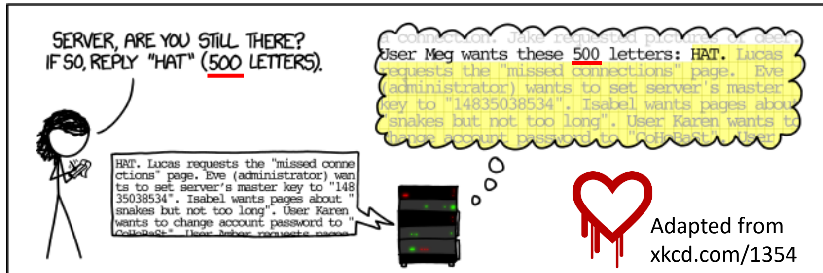
Heartbleed. OpenSSL bug that affected half a million web servers in 2014. A modified client sends a TLS Heartbeat containing an invalid (but encrypted) length field.
